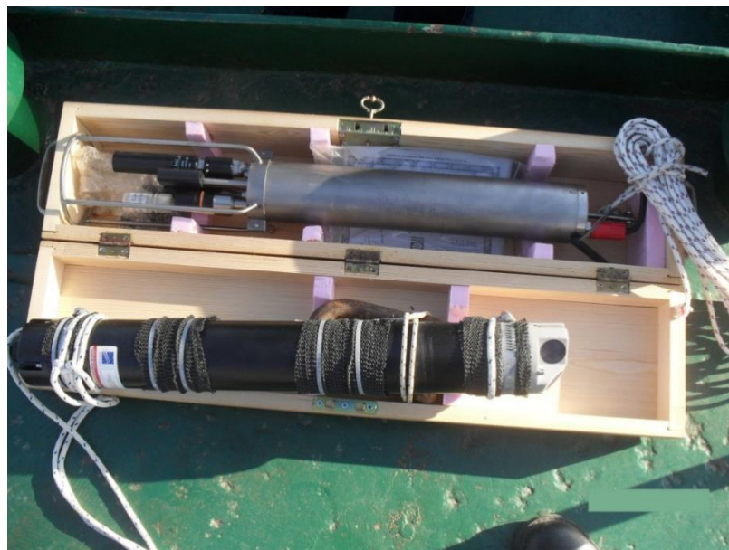
Figure 14: CTD and current meter used in the sampling provided by the Project coordinator
